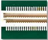
$\label{thm:linear} \mbox{Hidden bridge defect on connector joints can only be revealed by angle view camera.}$
