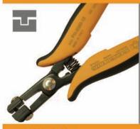
Special pliers designed to form the centre lead of TO 220 with 2.54mm pitch.
