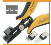
Special tool that enables TO220 component leads (7 leads) to be bent at a 90° angle in a single operation, in such a way that 2 - 4 - 6 leads will be 2.54 mm shorter than 1-3-5.
