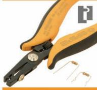
Forming pliers that cuts and C forms the component wire in one operation. Lenght setting is carried out by means of a sliding stop (A min 3 max 16).
