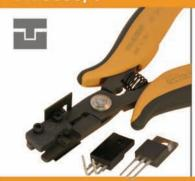
Special pliers that enables TO220 component leads to be bent at a 90° angle in a single operation, in such a way that the centre lead will be 2.54mm longer than the side leads.
