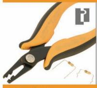
Pliers which forms the component wire in a C shape and cuts off the residual part. Residual component lead's length 3mm.
