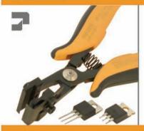
Special tool for a clean and flush cut at adjustable height from the surface of a pins line. It is possible to adjust the distance by a sliding foil (min. 1,5 max. 10 mm).
