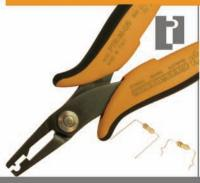
Pliers which forms the component wire in a C shape and cuts off the residual part. Residual component lead's length 4mm.
