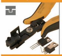
Special pliers that enables TO220 component leads to be bent at a 90° angle in a single operation, in such a way that the centre lead will be 2.54mm shorter than the side leads.
