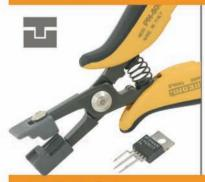
Special pliers that enables TO220 component leads to be bent at a 90° angle in a single operation, in such a way that the centre lead will be 3.81mm longer than the side leads.
