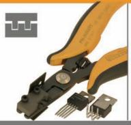
Special pliers that enables TO220 component leads (5 leads) to be bent at a 90° angle in a single operation, in such a way that 1-3-5 leads will be 2.54mm shorter than 2-4 leads.
