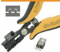
Special tool that enables TO220 component leads (5 leads) to be bent at a 90° angle in a single operation, in such a way that 2 - 4 leads will be 3.81 mm shorter than 1-3-5 leads.
