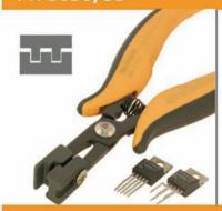
Special pliers designed to form the TO220 component leads (5 leads). It forms the 1-3-5 leads, 3mm pitch.
