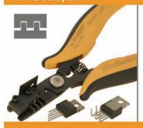
Special tool that enables TO220 component leads (5 leads) to be bent at a 90° angle in a single operation, in such a way that 2 - 4 leads will be 2.54 mm shorter than 1-3-5 leads.
