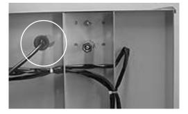
Mount the front cap (4) by placing it in the upper track. Bow the cap slightly and press it in the lower track.
