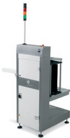
The basic unit of Single Magazine Handler.
