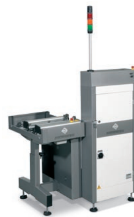
Single Magazine Handler with in feed / out feed conveyor • line loading with outfeed conveyor and PCB puller mechanics • line unloading with in feed conveyor with PCB pusher mechanics
