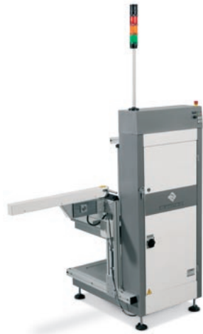
Single Magazine Handler with pusher mechanics for line loading.
